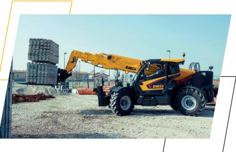
Icarus Dynamic, in the New Construction Range, is the vehicle that reaches great heights: it can extend **up to 18 meters**, guaranteeing **maximum stability** thanks to the proportionally controlled independent outriggers.
