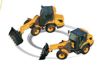
The vehicle overall dimension is always determined by the front or rear wheels, ensuring the operator that rear side will not hit while maneuvering.
