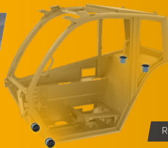
Front Silent Block with variable absorption
